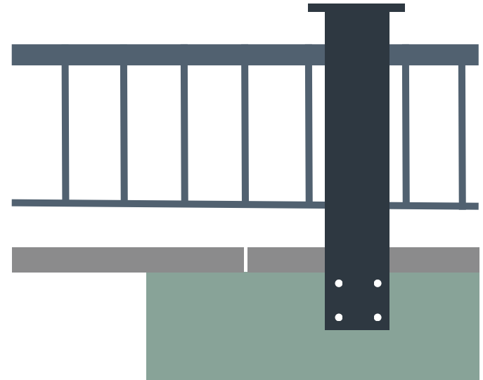
Side view - external joist*
